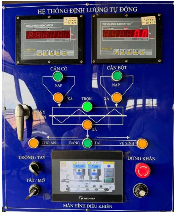
Fig. 9: Control screen of the proposed system.
